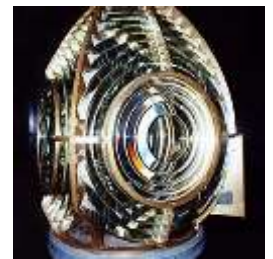
3 ½ order Fresnel Lens from DeTour Reef Light now on display in DeTour Passage Historical Museum
