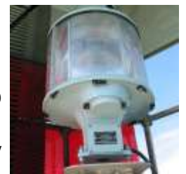
Six sided VRB-25 prior to removal from the DeTour Reef Light
